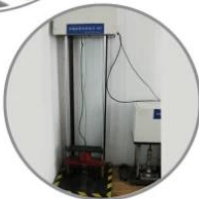
Impact Resistant Testing Machine
