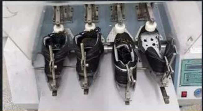
Flex Tester \geq 36,000 T
