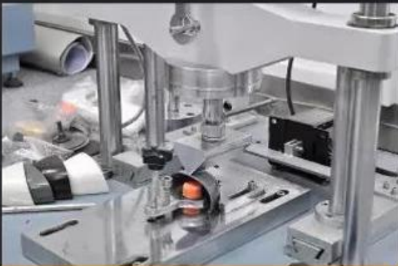
Toecap Test \geq 200 Joules
