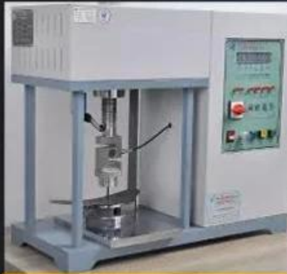
Midsole Test \geq 1200 Newtons
