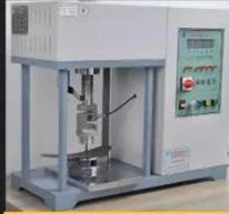
Midsole Test≥1200 Newtons
