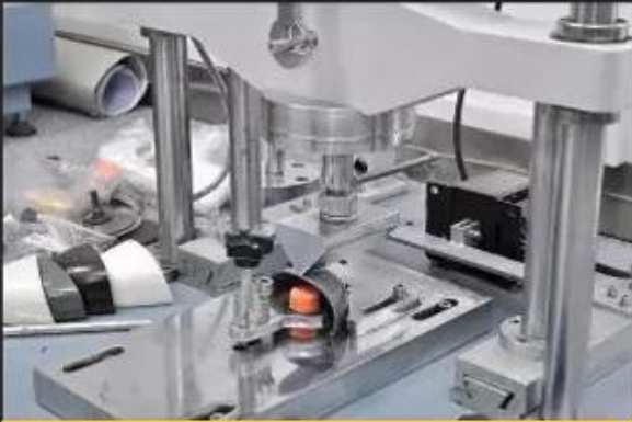
Toecap Test \geq 200 Joules
