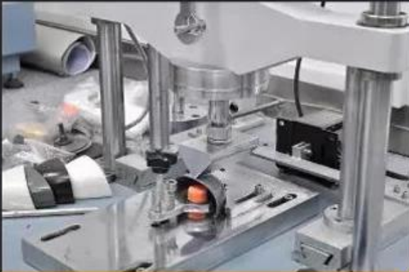
Toecap Test \geq 200 Joules
