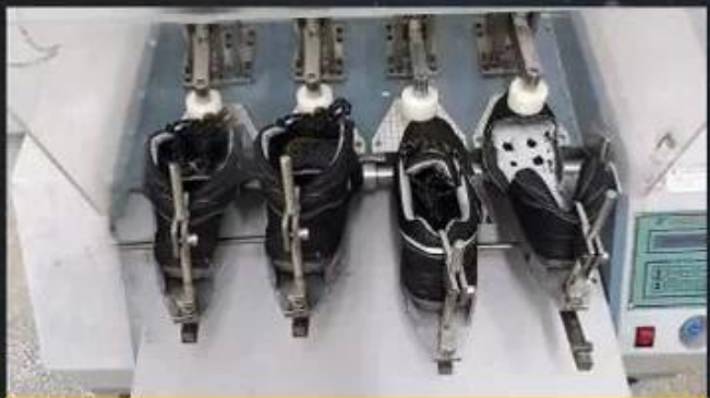
Flex Tester \geq 36,000 T
