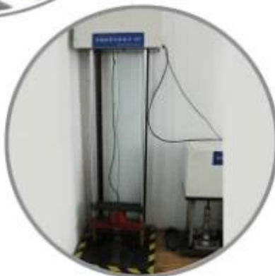
Impact Resistant Testing Machine
