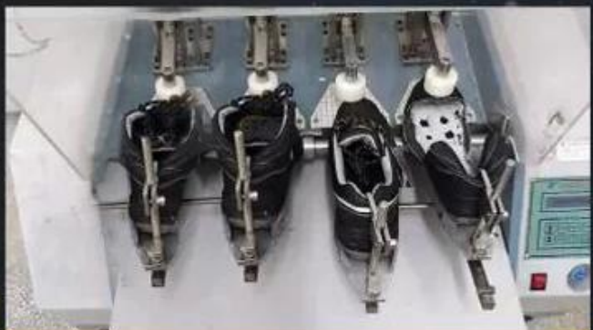
Flex Tester \geq 36,000T
