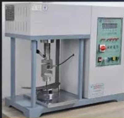
Midsole Test \geq 1200 Newtons
