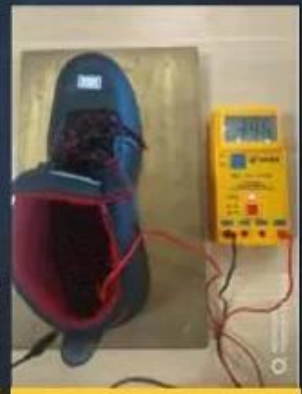
ESD Anti-Static Test
