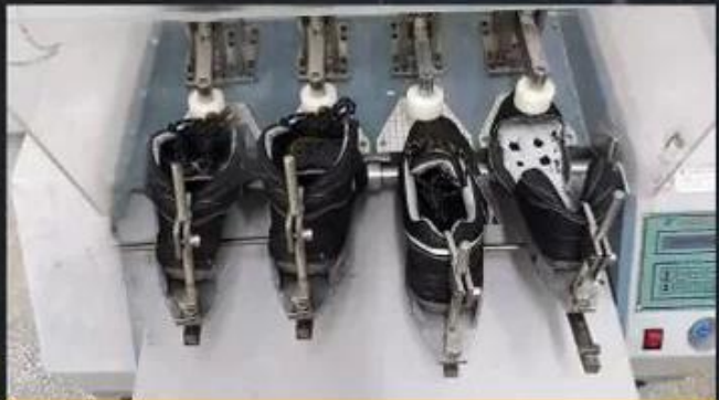
Flex Tester \geq 36,000T
