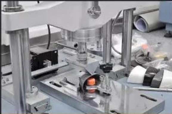
Toecap Test \geq 200 Joules
