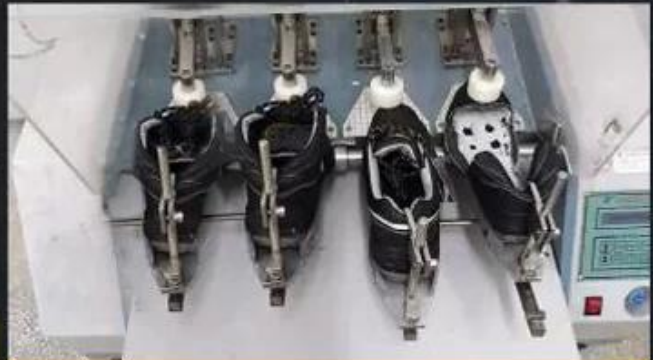
Flex Tester \geq 36,000 T
