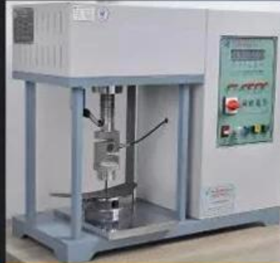
Midsole Test \geq 1200 Newtons
