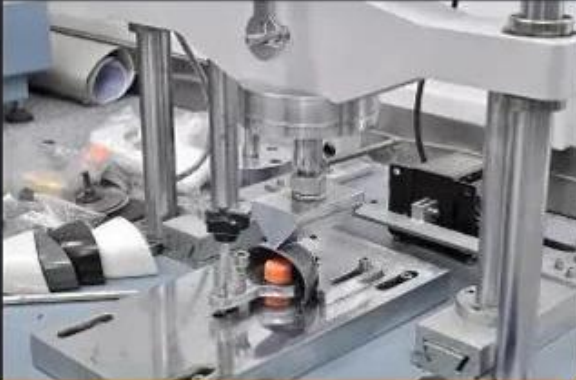
Toecap Test \geq 200 Joules
