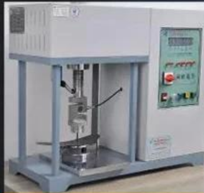
Midsole Test \geq 1200 Newtons
