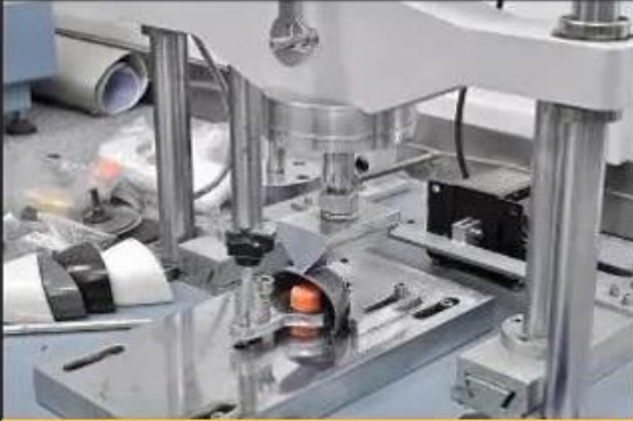
Toecap Test \geq 200 Joules
