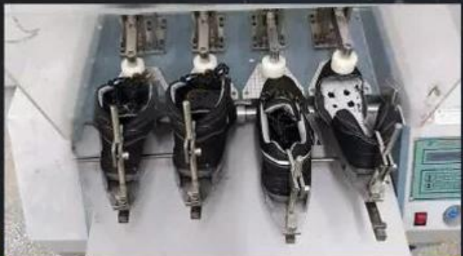
Flex Tester \geq 36,000 T
