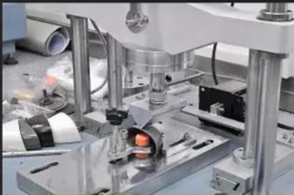
Toecap Test \geq 200 Joules
