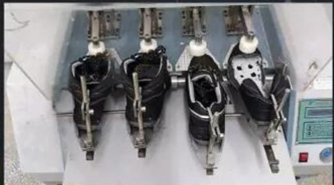
Flex Tester \geq 36,000 T
