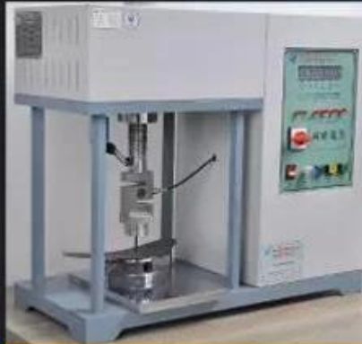
Midsole Test \geq 1200 Newtons
