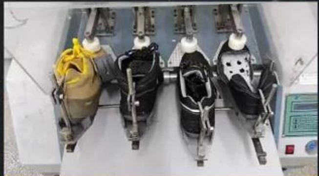
Flex Tester \geq 36,000 T
