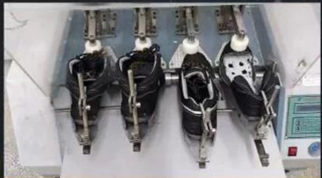
Flex Tester \geq 36,000 T
