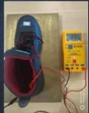
ESD Anti-Static Test
