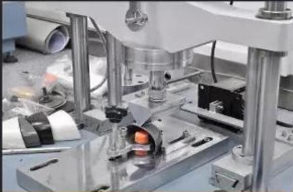
**Toecap Test  $\geq 200$  Joules**
