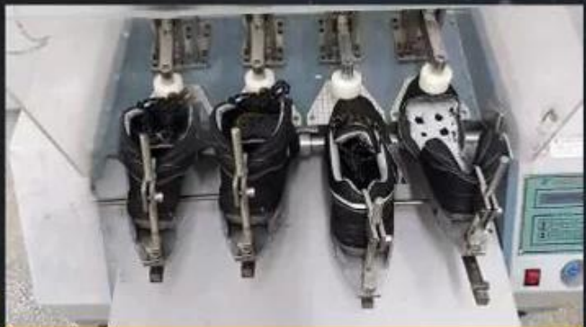
Flex Tester \geq 36,000T
