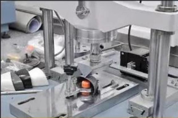
Toecap Test \geq 200 Joules
