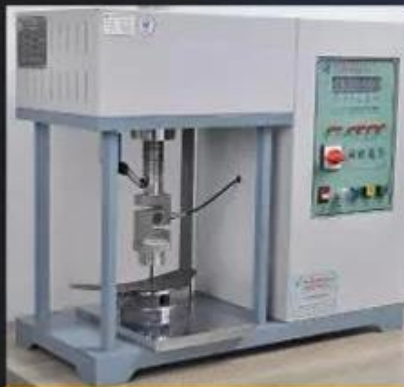
Midsole Test \geq 1200 Newtons
