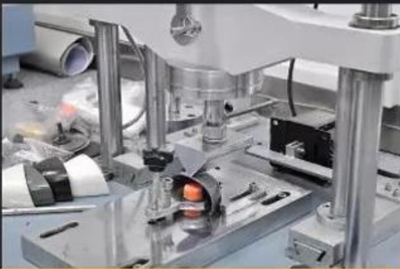
Toecap Test \geq 200 Joules
