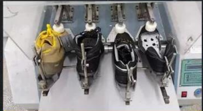
Flex Tester \geq 36,000 T
