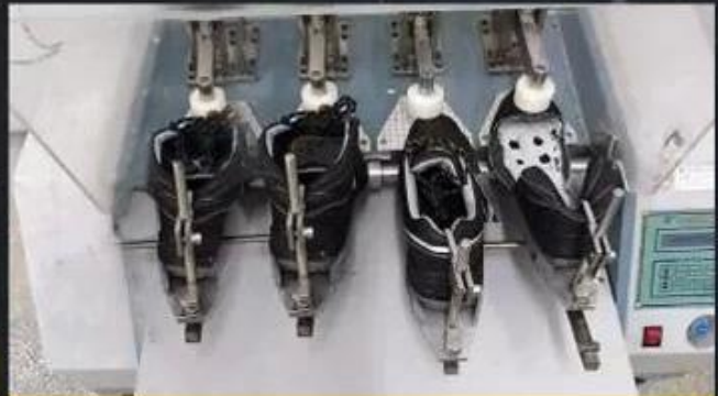
Flex Tester \geq 36,000 T
