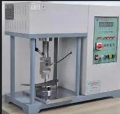
Midsole Test \geq 1200 Newtons
