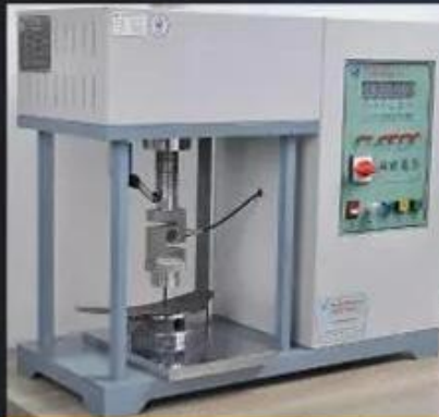
Midsole Test \geq 1200 Newtons
