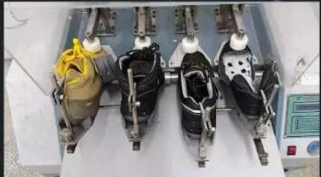
Flex Tester \geq 36,000 T
