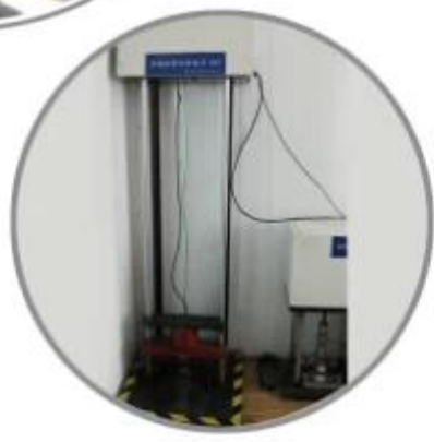
Impact Resistant Testing Machine
