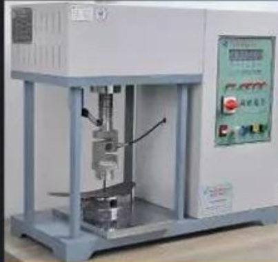
Midsole Test \geq 1200 Newtons
