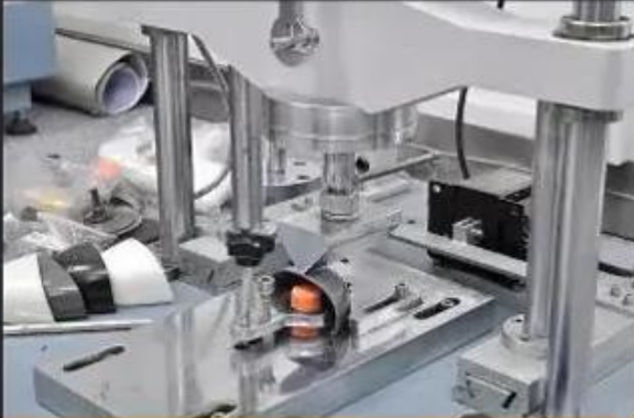
Toecap Test \geq 200 Joules
