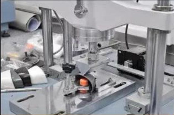
Toecap Test \geq 200 Joules
