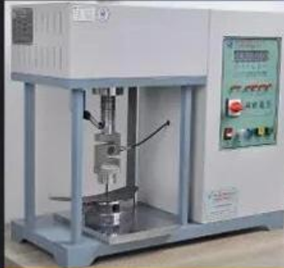
Midsole Test \geq 1200 Newtons
