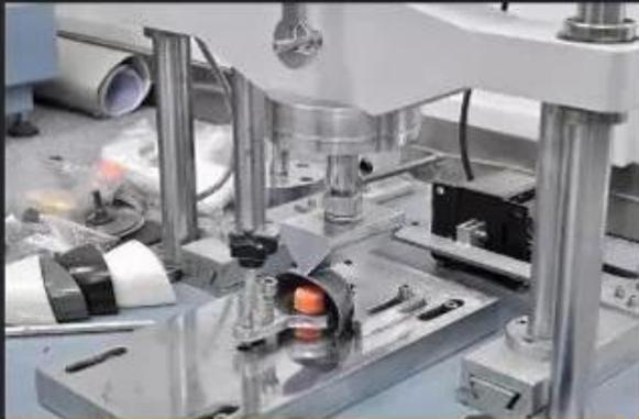
**Toecap Test  $\geq 200$  Joules**
