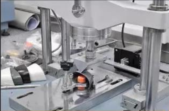
Toecap Test \geq 200 Joules
