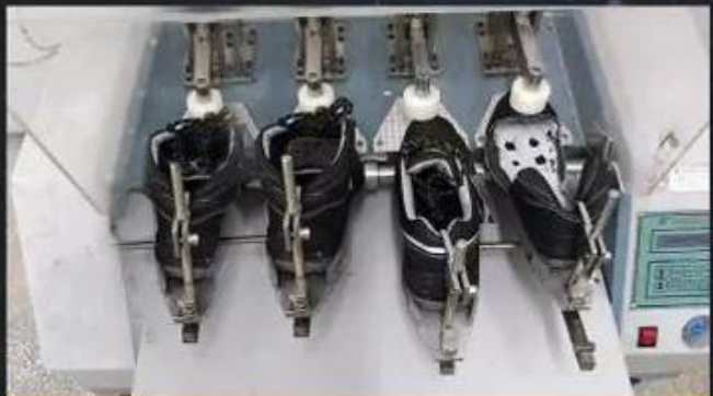
Flex Tester \geq 36,000 T
