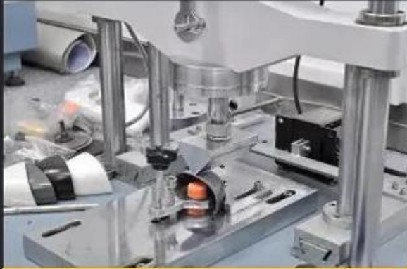
Toecap Test \geq 200 Joules
