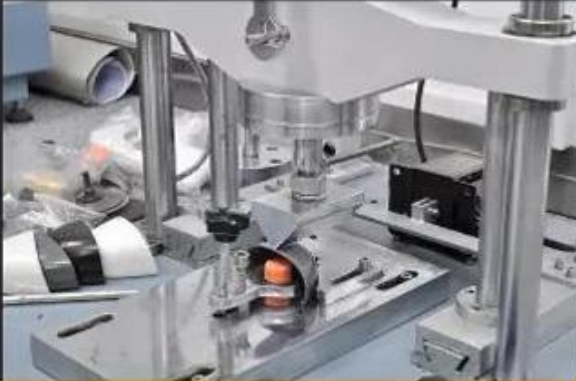
Toecap Test \geq 200 Joules
