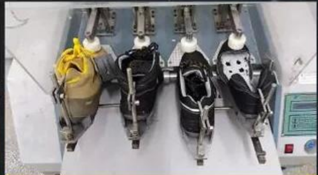
Flex Tester \geq 36,000 T
