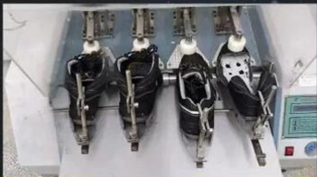
Flex Tester \geq 36,000T
