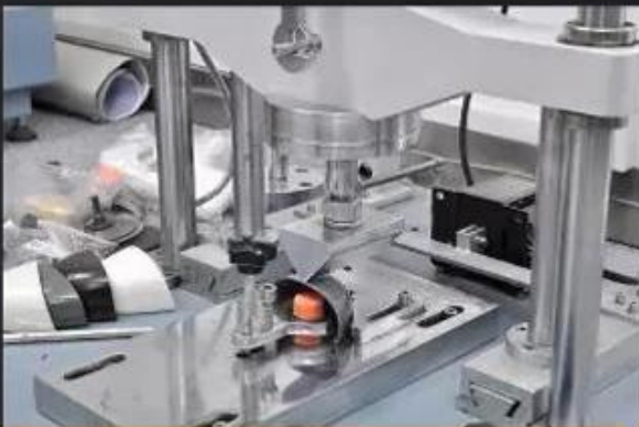
Toecap Test \geq 200 Joules
