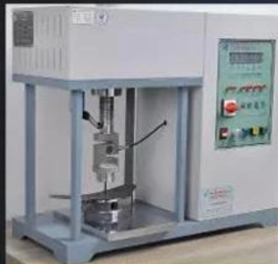
Midsole Test \geq 1200 Newtons
