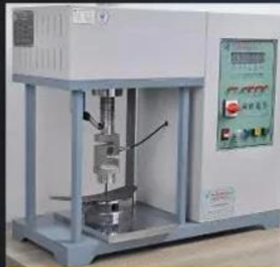
Midsole Test \geq 1200 Newtons
