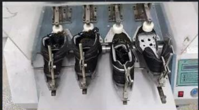
Flex Tester \geq 36,000 T
