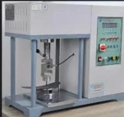
Midsole Test \geq 1200 Newtons
