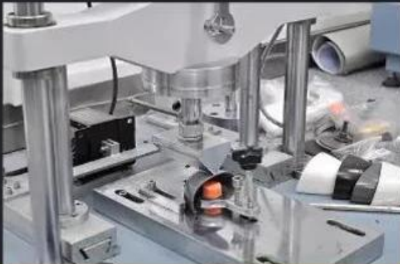
Toe cap Test \geq 200 Joules
