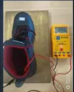
ESD Anti-Static Test
