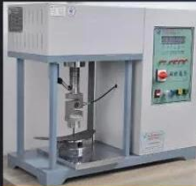
Midsole Test \geq 1200 Newtons
