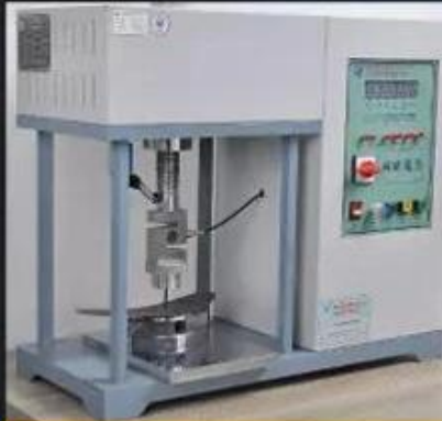
Midsole Test \geq 1200 Newtons
