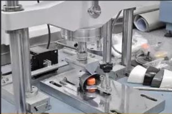
Toe cap Test \geq 200 Joules
