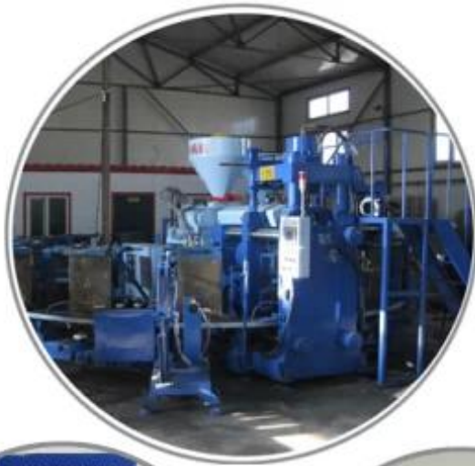
Automatic Injection Molding Machine
